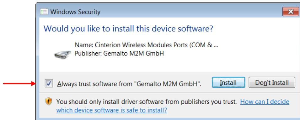
After the installation of the first device, go to ***Device manager, Action → Scan for hardware changes***.
